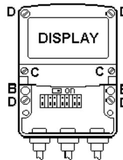
Install cable glands, conduit fittings or blanking plugs and terminate field wiring. If the instrument is about to be commissioned put the ON / OFF switch in the ON position . Finally replace the terminal cover and tighten the two 'A' screws.
