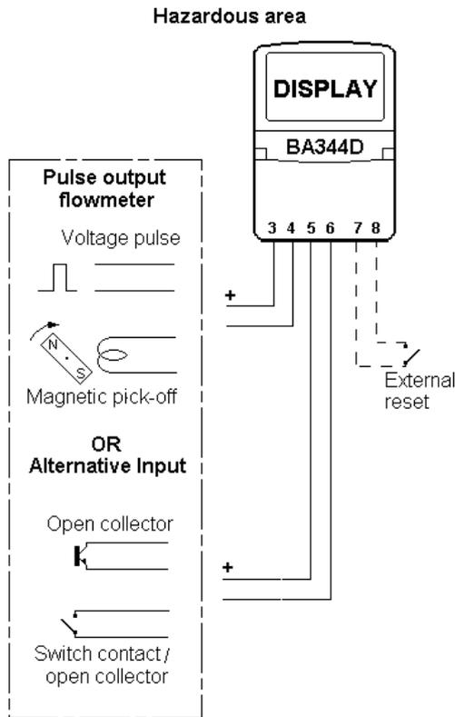
Fig 2 Stand alone operation within hazardous area
