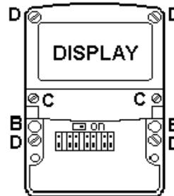
Secure the instrument to a flat surface with M6 screws through the two 'B' holes. Alternatively use a pipe mounting kit.
