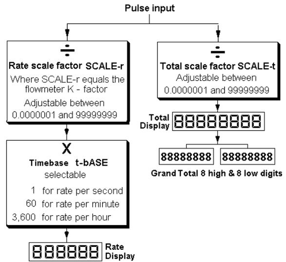
Fig 8 Calibration structure
