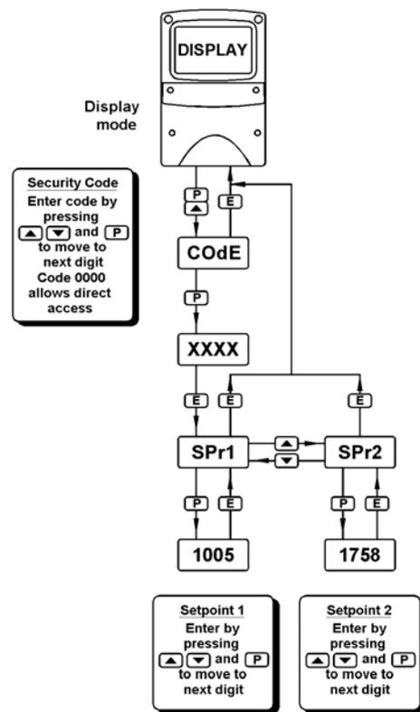
Fig 14 Setpoint adjustment from the display mode
