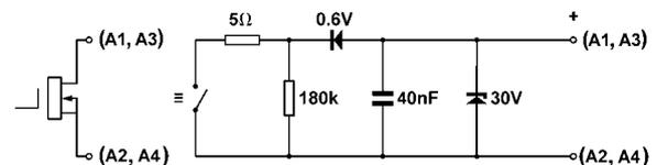
Fig 11 Equivalent circuit of each alarm output
