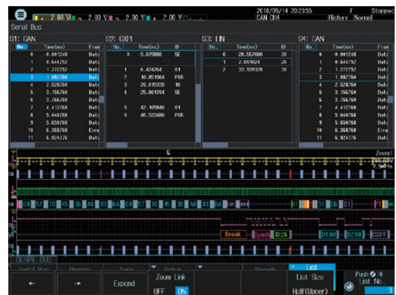
Four bus decode and list display
