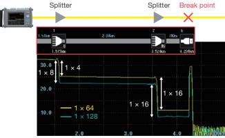
Measurements over a 128 and 64-port splitter
