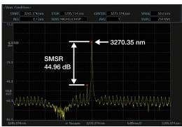
Measurement example of 3270 nm DFB-LD (Res: 0.1 nm, Span: 50 nm)
