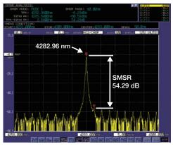
Measurement example of 4.3 µm DFB laser (Res: 0.2 nm, Span: 50 nm)
