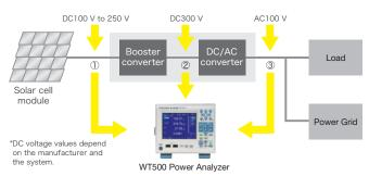
Overview of a Photovoltaic Inverter Evaluation
