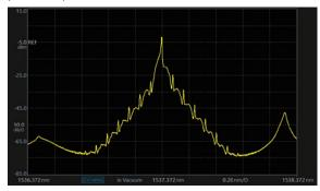
Modulated spectrum of 10 G optical transceiver
