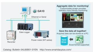
GA10 is a PC based software package that acquires data from multiple devices – such as power meters (WT series), recorders, and data loggers. Connected PCs can monitor real time and historical data, which can be stored on a PC hard drive.
