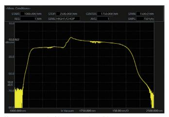
Measurement example of 2  $\mu m$  supercontinuum light source (by use of Extended model)
