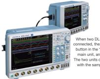
When two DLM5000HD/5000 series models are connected, the one that you press the "Connect" button in the "DLMsync" menu on becomes the main unit, and the other becomes the sub unit. The two units capture waveforms simultaneously with the sampling clock and trigger of the main
