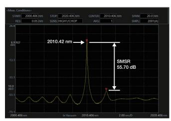
Measurement example of 2010 nm DFB-LD (Res: 0.05 nm, Span: 20 nm)
