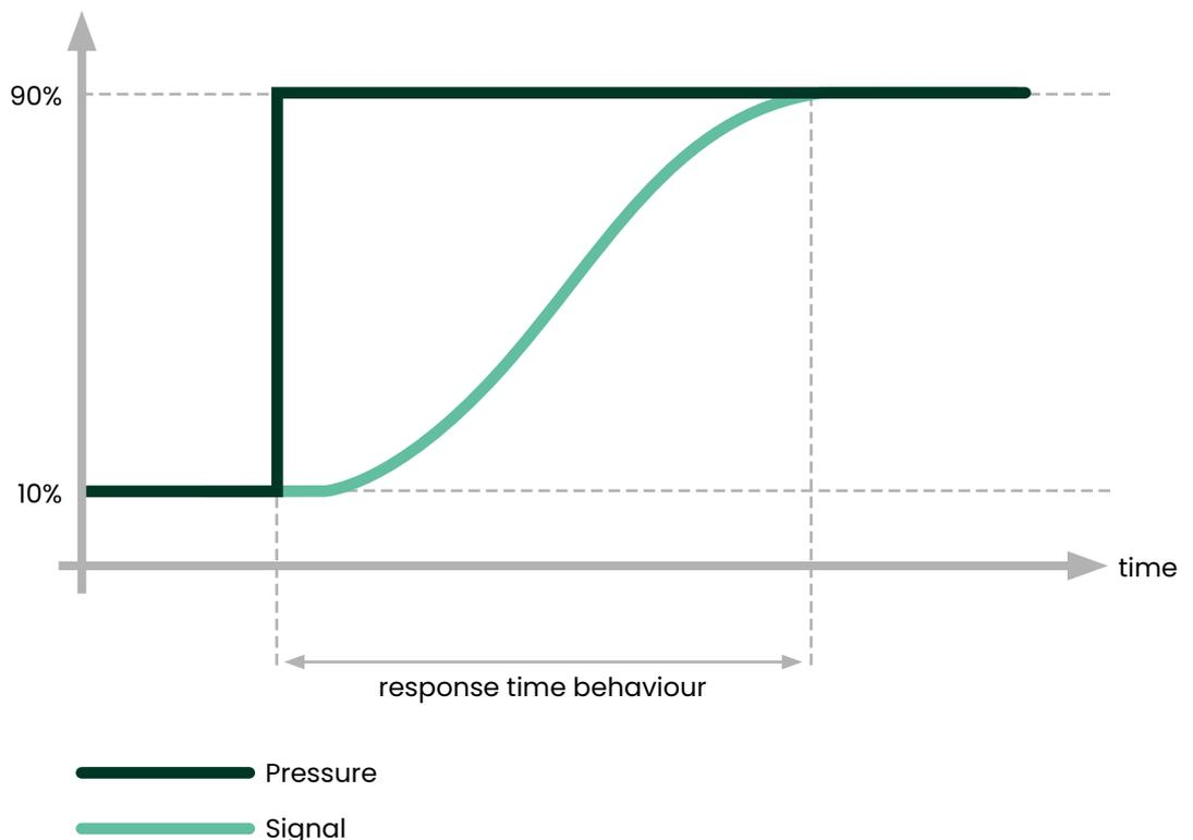
When taking readings at a speed approaching the response time it is possible to generate very large errors.
